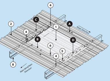
Typical, Single Panel, Single Span Mid-Field Detail Figure 25
