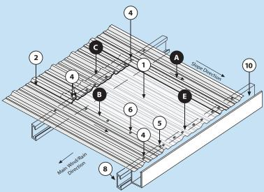
Typical Bottom End SunSky Detail (with or without gutter) Figure 26
